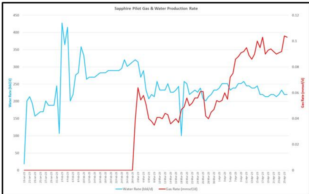
Figure 1: Graph showing gas rate increasing with time as water rate stabilises.
